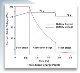
Three stage charging is recommended by battery manufacturers. It delivers the most amp-hours of charge in the shortest amount of time. A current sensor regulates 1st stage battery current at 90 amps regardless of other loads. The higher voltage 2nd stage fully converts battery plate lead sulfate to prevent battery sulfation. The lower voltage 3rd stage maintains full charge and reduces electrolyte loss on long runs.
