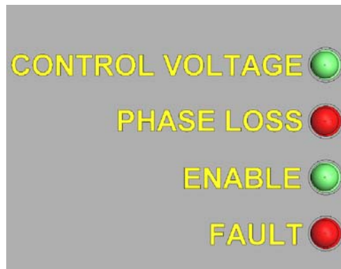
Figure 2—Front Panel LED Status Indicators
