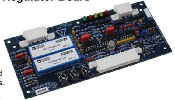
**Soft-Start and Soft-Stop:** The soft-start circuit ramps the gate delay command voltage input to the firing board up to the preset level in approximately 2 seconds; the soft-stop ramps the command down in a similar fashion. Other soft-start times may be specified.
