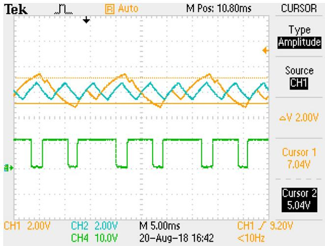
Figure 2. Phase Loss Circuit Signals – Phase Loss
