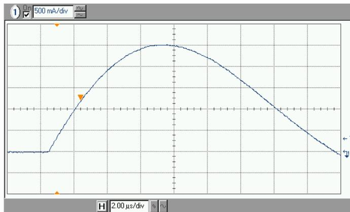
Figure 7. Initial pulse profile detail (Into 1Ω).
