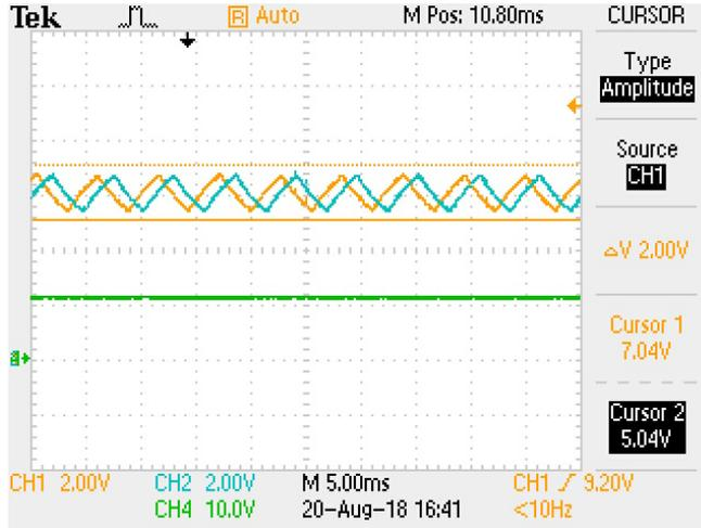
Figure 1. Phase Loss Circuit Signals – No Phase Loss<sup>4</sup>
