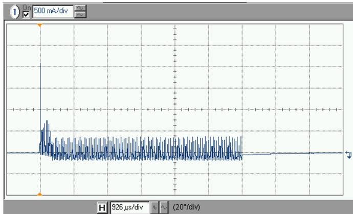
Figure 6. 120° Gate Pulse Profile (Into 1Ω).
