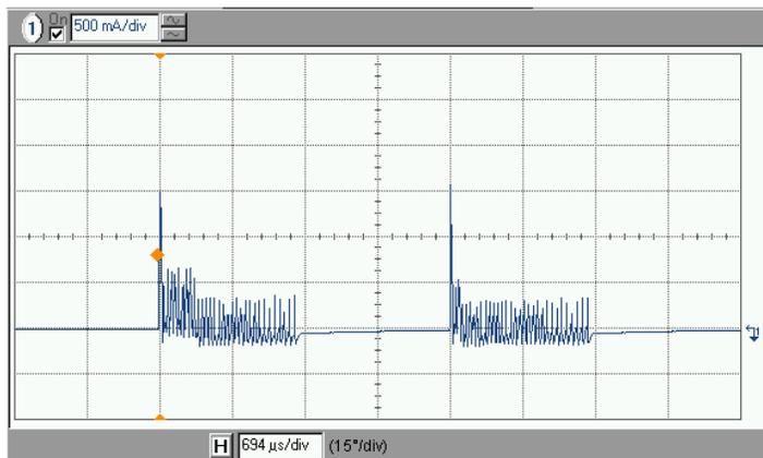
Figure 5. 2-30° Gate Pulse Profile (Into 1Ω)<sup>5</sup>
