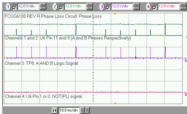
Figure 2. Phase Loss Circuit Signals – Phase Loss Channels: 1. Digital A Phase Reference Signal, U6 P11 2. Digital B Phase Reference Signal, U6 P9 3. A and B logic signal, TP8 4. \overline{PL} Signal, U6 P1
