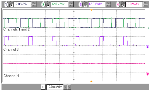
Figure 2. Phase Loss Circuit Signals – No Phase Loss 4 Channels: 1. Digital A Phase Reference Signal, U4 P11 2. Digital B Phase Reference Signal, U4 P9 3. A and B logic signal, TP9 4. \overline{PL} Signal, U4 P1
