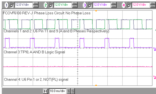
Figure 1. Phase Loss Circuit Signals – No Phase Loss 4
